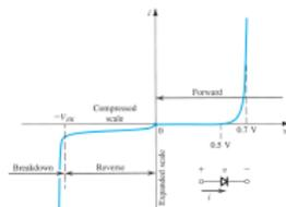
FIG 3. A detailed  $i-v$  characteristic of a silicon junction diode.
