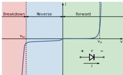
FIG 4. I-V characteristics of a p-n junction diode
