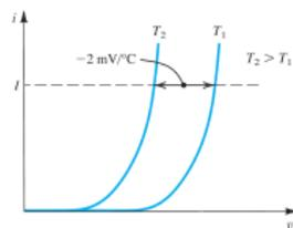
**FIG 2.** Diode temperature dependence
