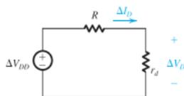
FIG 5. A nonlinear diode circuit can be replaced by a linear resistor circuit under the small signal approximation
