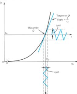
FIG 7. The diode small-signal model
