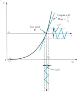
FIG 3. The diode small-signal model.
