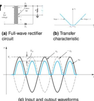
FIG 3. Full-wave rectifier utilizing a transformer with a center-tapped secondary winding
