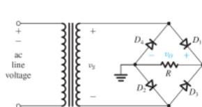
(a) Bridge rectifier circuit
