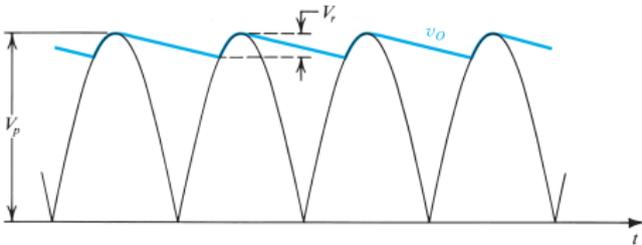
FIG 12. Waveforms in the full-wave peak rectifier.
