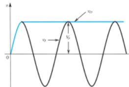
(b) Input and output assuming an ideal diode
