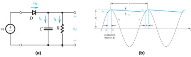
FIG 11. Peak rectifier with  $v_i > 0$  for an ideal diode
