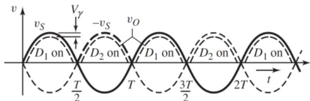
**FIG 4. Full-wave rectifier working principle**
