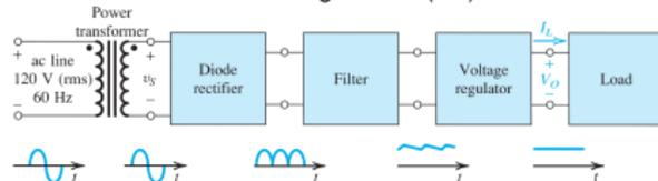
FIG 1. Block diagram of a dc power supply
