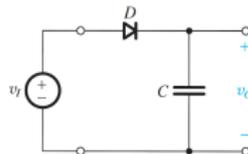
(a) diode with a capacitor
