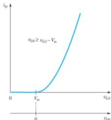
FIG 9. The  $i_D$  vs  $V_{GS}$  characteristic in the saturation region. The  $i_D$  vs  $V_{GS}$  characteristic can be obtained by simply relabeling the horizontal axis, that is, shifting the origin to the point  $V_{GS} = V_{tn}$
