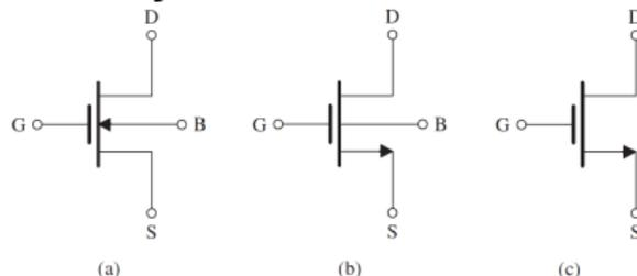
FIG 1. Common MOSFET circuit symbols
