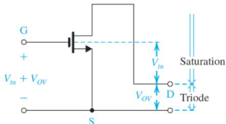
FIG 5. The relative levels of the terminal voltages of the enhancement NMOS transistor for operation in the triode region and in the saturation region. Note that the operation mode depends on the drain-source voltage
