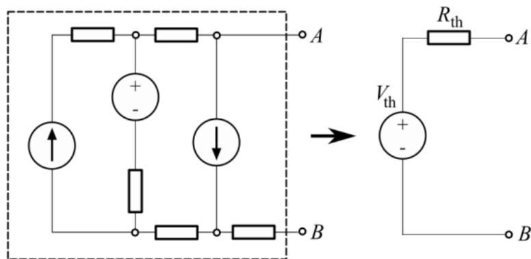
**FIG 1. Thevenin model of a circuit<sup>2</sup>**
