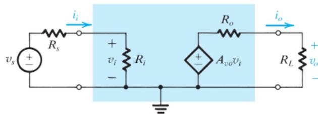
FIG 3. Voltage amplifier with input signal source
