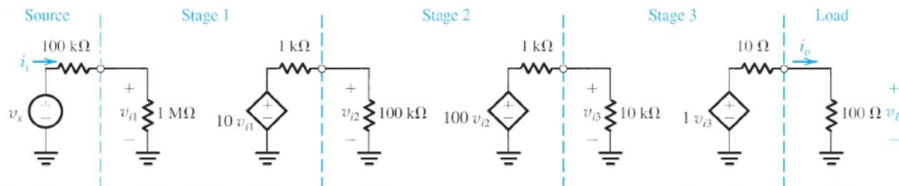
**FIG 4. Three-stage amplifier**
