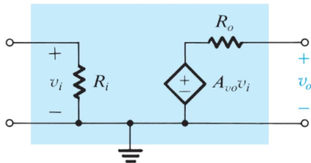
FIG 2. Circuit model for the voltage amplifier
