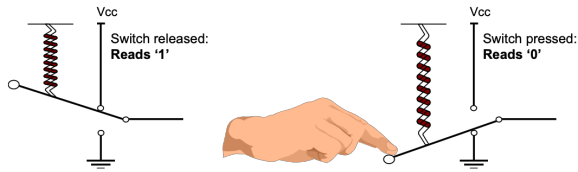
FIG 24. With a pull-up resistor, the input pin will read a high state when the button is not pressed.
