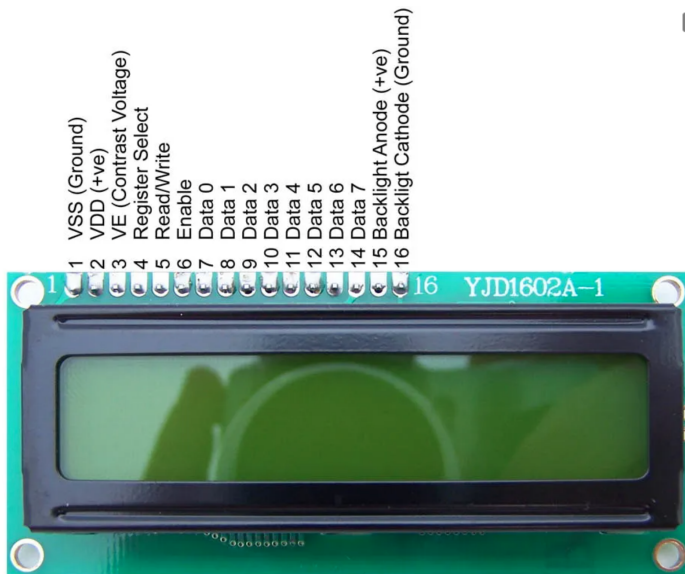
FIG 26. A 16×2 LCD based on HD44780
