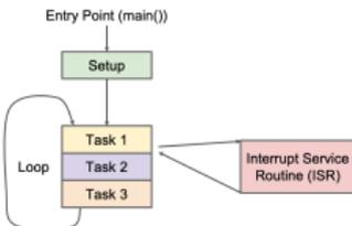
FIG 1. Architecture without an RTOS
