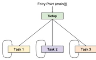
FIG 2. Architecture with an RTOS
