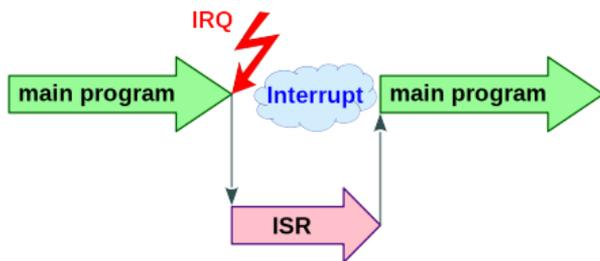
FIG 1. Principle of an interrupt
