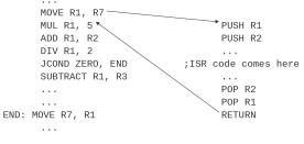
FIG 2. Example of assembly code of ISR
