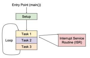
FIG 1. Architecture without an RTOS
