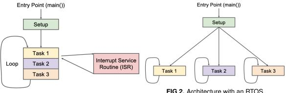
FIG 1. Architecture without an RTOS
