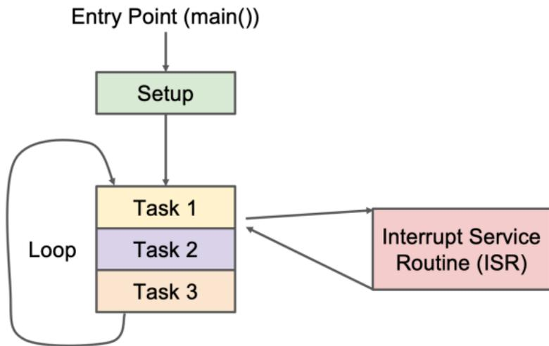
**FIG 1.** Architecture without an RTOS
