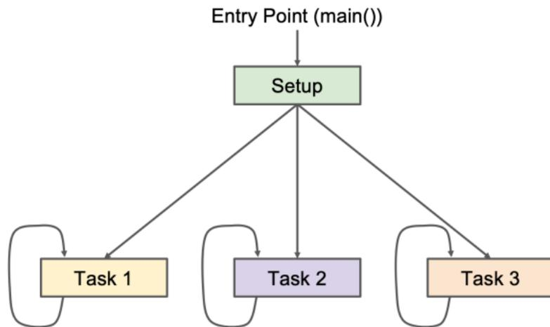
**FIG 2.** Architecture with an RTOS
