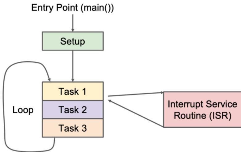
**FIG 1.** Architecture without an RTOS
