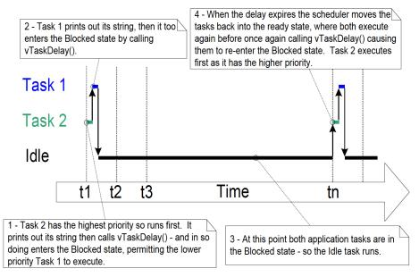
FIG 7. The execution sequence when the tasks use vTaskDelay()
