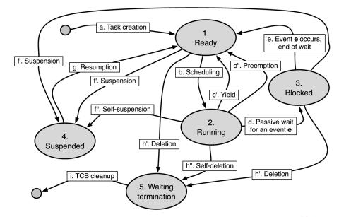
FIG 4. Task state diagram in the FREERTOS operating system.<sup>14</sup>
