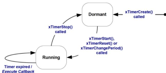
FIG 10. Auto-reload software timer states and transitions
