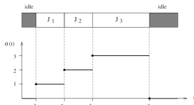
FIG 1. Schedule obtained by executing three tasks J_1 , J_2 , and J_3
