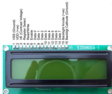
FIG 26. A 16×2 LCD based on HD44780
