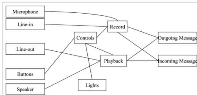
FIG 1. Simplified class diagram of the office telephone
