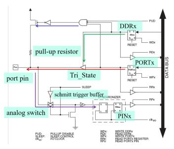
**FIG 6.** The ports are bi-directional I/O ports with optional internal pull-ups.
