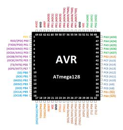
FIG 7. ATMEGA128 pin out
