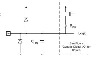
FIG 5. AVR I/O Pin Equivalent Schematic The AVR I/O ports are the path to the outside world. The ports has protection diodes and programmable pull-up resistor
