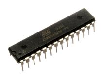
FIG 2. ATmega328P in dual in-line package
