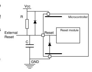
FIG 12. Recommended Reset Pin connection.
