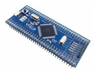
**FIG 8.** ATMEGA128 Module with Arduino bootloader
