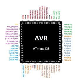
FIG 11. ATMEGA128 pin out
