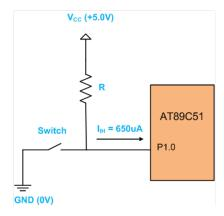
FIG 22. Switch interfacing
