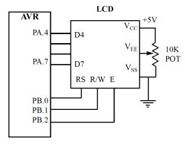
FIG 30. LCD Connections Using 4-bit Data
