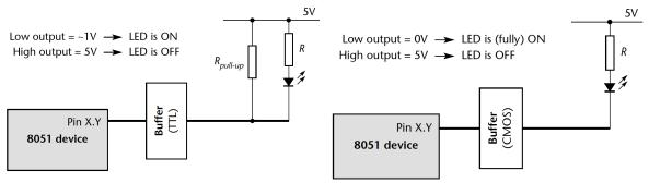
FIG 5. Using a TTL buffer
