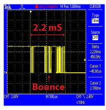
FIG 25. Example of a push-button switch being pressed, as seen on the oscilloscope:
