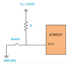
FIG 21. Switch interfacing
