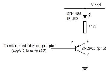
FIG 13. Driving an IR LED via a transistor (PNP) driver
