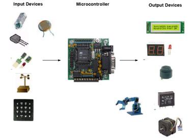
FIG 1. Micro-controllers are used to communicate with other devices, such as sensors, motors, switches, keypads, displays, memory and even other micro-controllers. In a very simplistic form, a micro-controller system can be viewed as a system that reads from (monitors) inputs, performs processing and writes to (controls) outputs.
