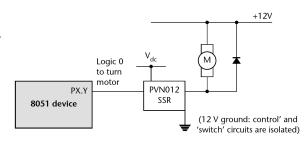
FIG 20. Open-loop DC motor control using a solid-state relay
