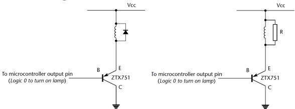
FIG 10. Protecting transistors against inductive kick with a diode
