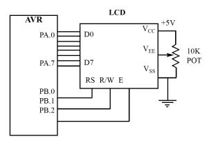
FIG 28. LCD Connections for 8-bit Data
