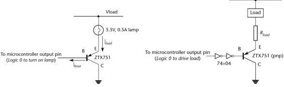
FIG 8. A PNP transistor driving a lamp.
