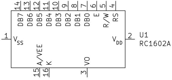
FIG 27. Schematic symbol for a 16×2-character LCD
