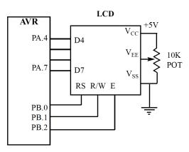
FIG 29. LCD Connections Using 4-bit Data
