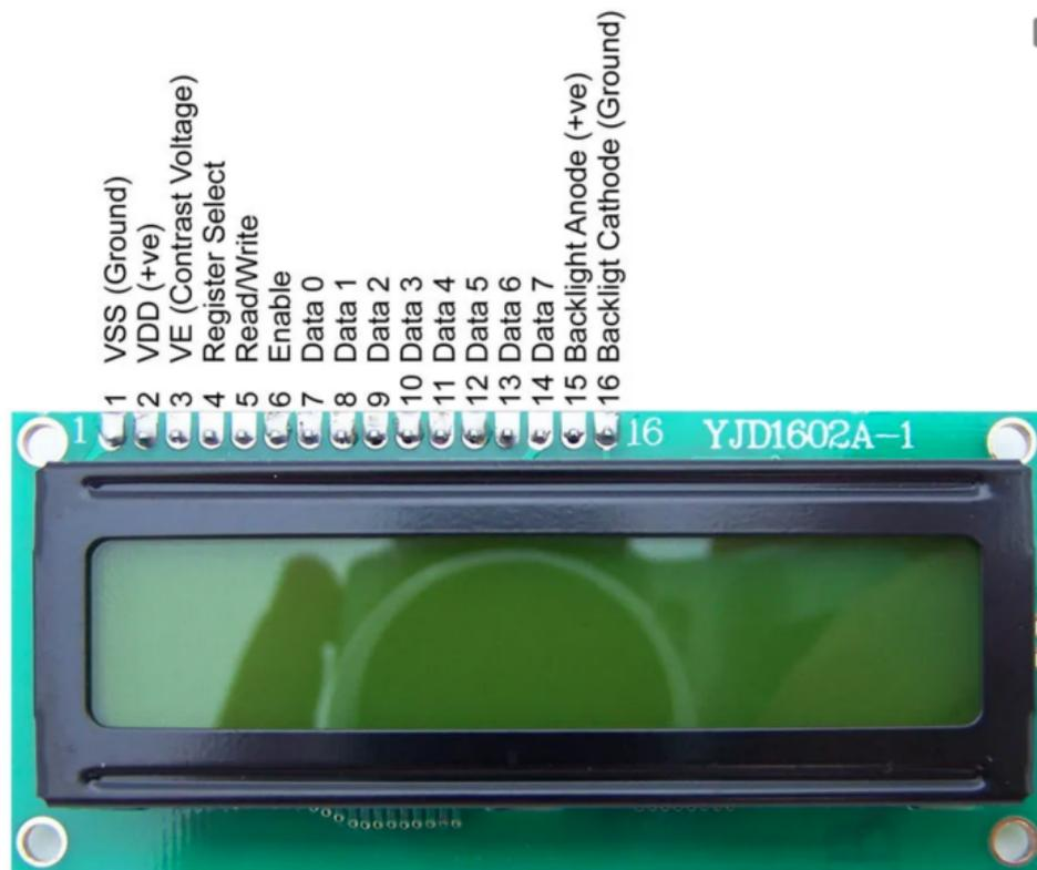
**FIG 26.** A 16×2 LCD based on HD44780
