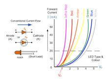
FIG 3. Light Emitting Diodes I-V Characteristics
