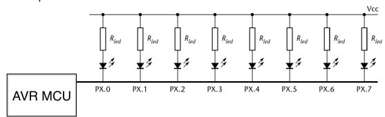
■ This approach won't work because each I/O pin can sink or source a maximum current of 40mA. Although each pin can sink or source 40mA current, it must be ensured that the current sourced or sunk from all the ports combined, should not exceed 200mA.
