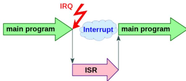
**FIG 1.** Principle of an interrupt
