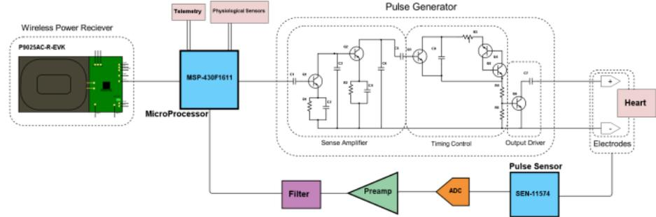
**FIG 1.** A pacemaker is a small, battery-operated device. This device senses when your heart is beating irregularly or too slowly. It sends a signal to your heart that makes your heart beat at the correct pace. In general, a heart pacemaker contains a small micro-controller and electrodes that connect the heart to the generator. The electrodes carry the electrical message to the heart. A defective pacemaker can cause more harm than good
