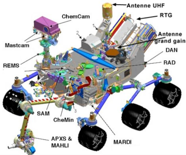
**FIG 5.** Instrumentation of the Mars Rover
