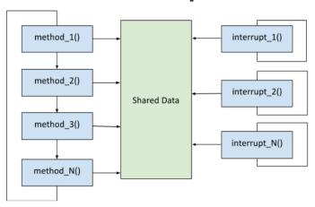
FIG 5. Round Robin with Interrupts<sup>1</sup>
