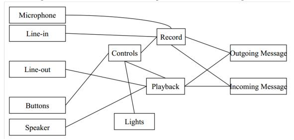
FIG 1. Simplified class diagram of the office telephone
