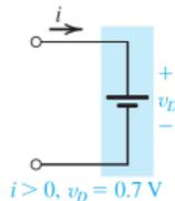
(c) the resulting model of the forward-conducting diodes
