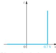
(b) approximating by a constant voltage (usually  $V_D = 0.7V$ )
