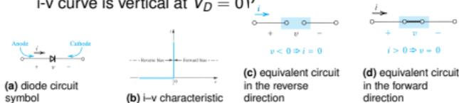
FIG 5. The ideal diode model
