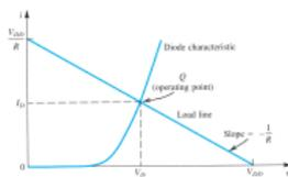
**FIG 3.** Illustration of the graphical analysis method using the exponential diode model
