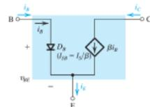
FIG 11. Model 4 —Current-controlled current-source
