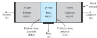
FIG 1. A simplified structure of the npn transistor
