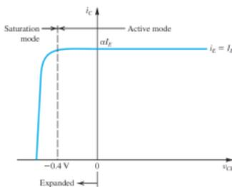
FIG 12. The  $i_C$  vs  $v_{CB}$  characteristic of an npn transistor fed with a constant emitter current  $I_E$ . The transistor enters the saturation mode of operation for  $v_{CB} < -0.4V$ , and the collector current diminishes.
