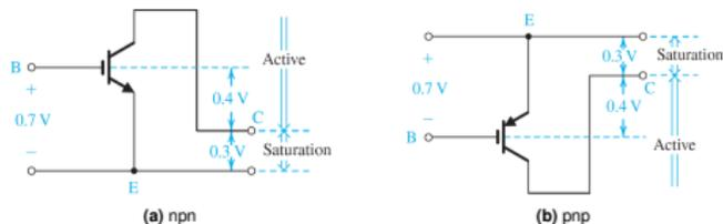
**FIG 17.** Graphical representation of the conditions for operating the BJT in the active mode and in the saturation mode.
