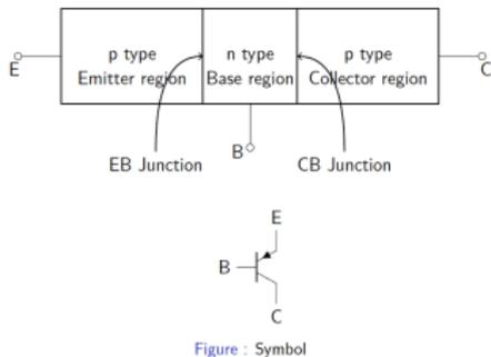
FIG 4. Simplified structure of a pnp BJT transistor
