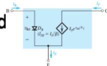
FIG 10. Model 3—A voltage-controlled current source
