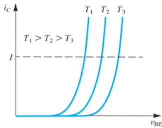
FIG 15. Effect of temperature on the  $i_C$  vs  $v_{BE}$  characteristic. At a constant emitter current (broken line),  $v_{BE}$  changes by  $-2mV^{\circ}C^{-1}$
