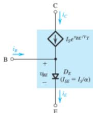
FIG 8. Model 1—A nonlinear voltage-controlled current source.
