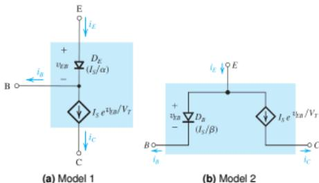
**FIG 16.** Two large-signal models for the pnp transistor operating in the active mode.
