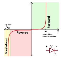
FIG 10. The I-V relationship of a real diode<sup>2</sup>
