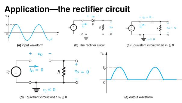
FIG 14. A half wave rectifier allows one half-cycle of an AC voltage waveform to pass, blocking the
