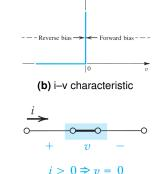
(c) equivalent circuit in the reverse direction
