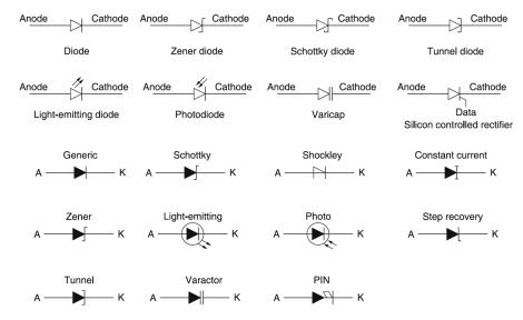
FIG 8. Various types of diodes and their schematic symbols<sup>2</sup>
