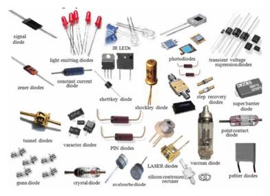
FIG 7. Various types of diodes<sup>1</sup>
