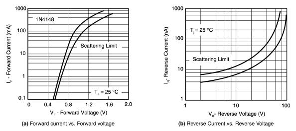
**FIG 12.** Typical behaviors of 1N4148 diode at  $T = 25 \degree C$
