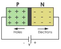
FIG 4. n-types and p-type arrangement in a diode
