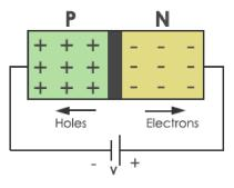
FIG 6. n-types and p-type arrangement in a diode
