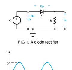
FIG 2. output of the rectifier
