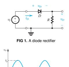
FIG 2. output of the rectifier
