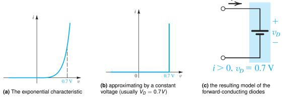
FIG 4. Development of the diode constant-voltage-drop model:
