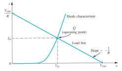
**FIG 3.** Illustration of the graphical analysis method using the exponential diode model
