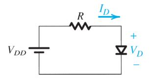
FIG 2. Illustrative diode circuit
