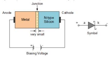
Schottky diodes are used in rectification, signal conditioning and switching, through to TTL and CMOS logic gates due to their low power and fast switching speeds.
