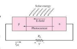
FIG 4. A pn junction solar cell connected to load
