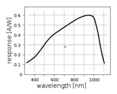
(b) Response of a photo diode vs wavelength of the incident light
